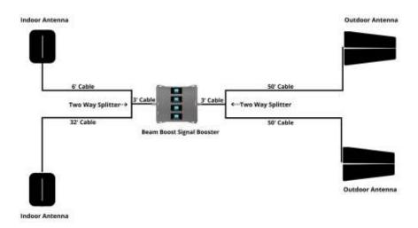
**TIP:** You can use the included cable however you like, as long as you maintain the distance between the indoor and outdoor antennas, i:e (You can use a 50' outdoor cable with an indoor antenna, Additionally you can also use one' cable to connect both outdoor antennas using a splitter at the outside end)
