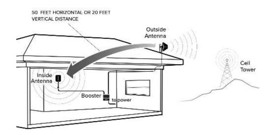
**Note:** The outside antenna must be at least **50 feet horizontal OR 20 feet vertical** from the inside antenna for best performance. Make sure the inside antenna and outside antennas are set up so they are **facing away** from each other.
