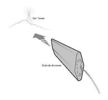
NOTE: **Dual outdoor antennas** can be pointed to one network carrier for better gain, and if you wish to use **two cell networks**, point each outdoor antenna towards both cell towers.
